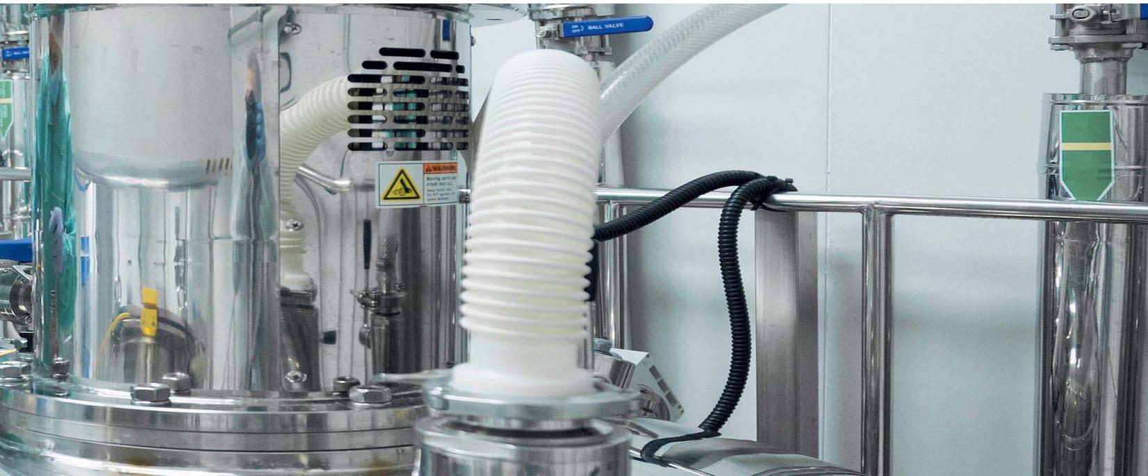
In pharmaceutical and chemical processing, the requirements for hygiene are particularly high. Hazards due to contamination with harmful substances, germs or microorganisms must be reliably excluded at all times. The housings of the monos easy clean can be made of **V2A** or **V4A stainless steel** and are therefore resistant to a wide range of chemicals.
