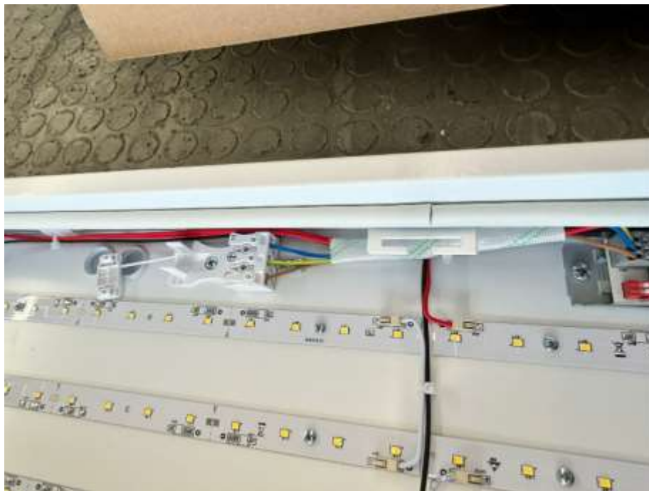
Photo 6. Electrical connections of the luminaire
