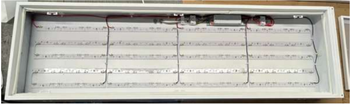
Photo 3. Internal view of the luminaire(Model 005.0001.6450)
